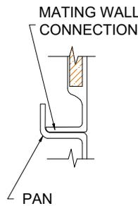
**DETAIL PJ - SCALE: 3" = 1'-0" PAN JOINT DETAIL**
