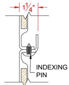
**DETAIL WJ - SCALE: 3" = 1'-0" WALL JOINT DETAIL**
