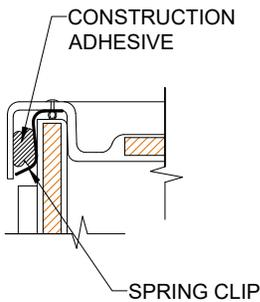
**DETAIL CD - SCALE: 3" = 1'-0" CORNER DETAIL**
